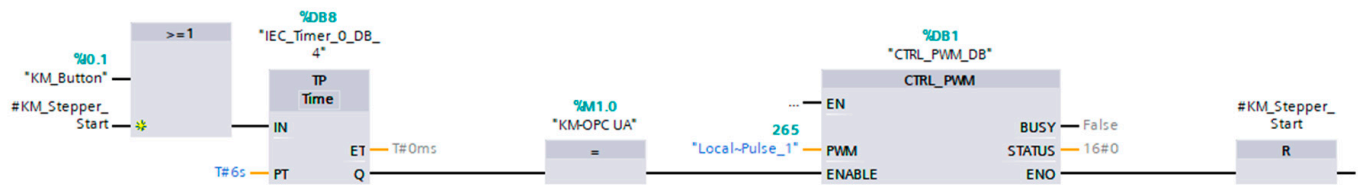
Figure 5. PLC programming of the loading device (KM) to release the beads.
