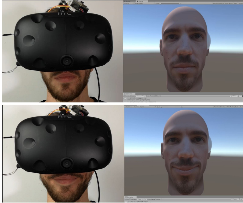
Figure 5.21.: In addition to eyebrow tracking, the system can track other expressions, such as a grin, with two sensors inserted into the foam on the cheeks. When grinning, the person's cheeks exerted a clearly measurable pressure on the sensors in the lower part of the foam. The pressure sensor approach was not pursued further because it was too susceptible to tracking errors during head movements. Image credits by Juan Schupp.
