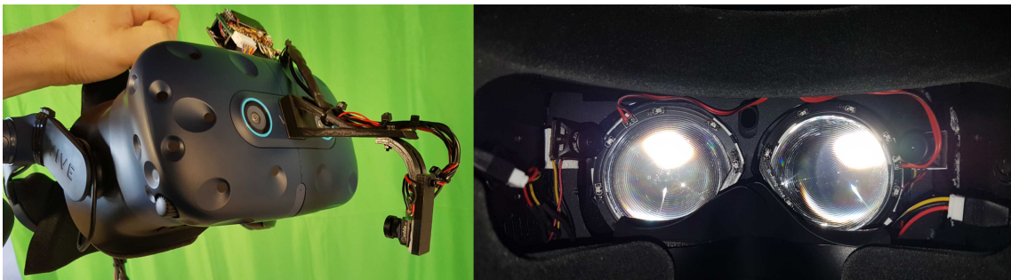
Figure 5.1.: To expand and improve the face tracking capabilities of an off-the-shelf eye-tracking HMD, we added three miniature IR sensors/cameras to it. Two of these sensors are used to track the movement of the eyebrows (right), while the remaining sensor focuses on the lower part of the face (left).
