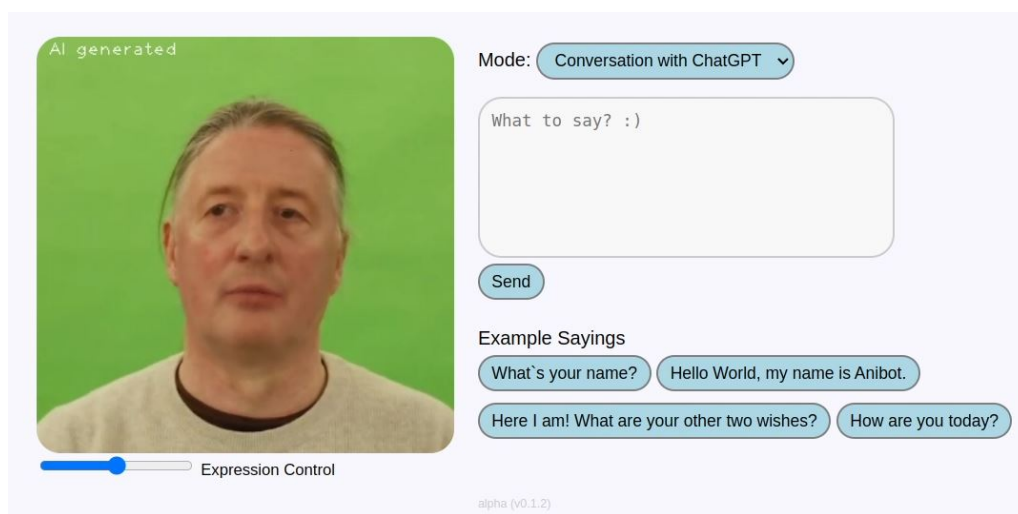
Figure 8.11.: Broader impact and use cases of our pipeline: With the use of ChatGPTs API and the combination with a Text-to-Speech service, our system is able to provide an interactive virtual assistance with a face. The right side of the image shows the GUI of our experiment in a web browser.
