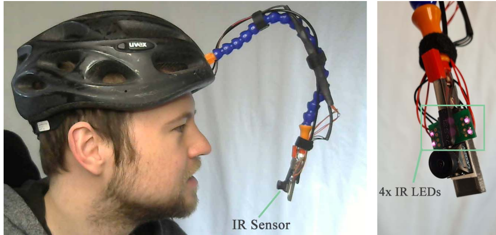
Figure 5.9.: Data acquisition using the "training mount": A bicycle helmet was modified by adding a mount with 4 infrared LEDs and a modified RGB sensor with an infrared band-pass filter instead of an RGB filter.
