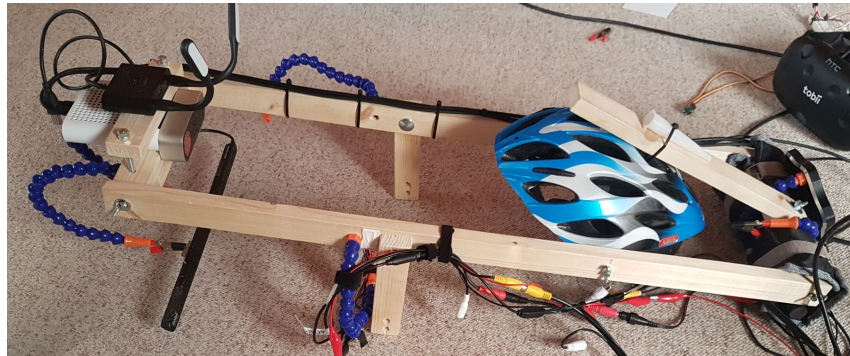
Figure 7.5.: A Tobii 4C eye tracker was used to reliably track the user's gaze. The eye tracker (black thin bar) is mounted below the Azure Kinect on the left side of the image.
