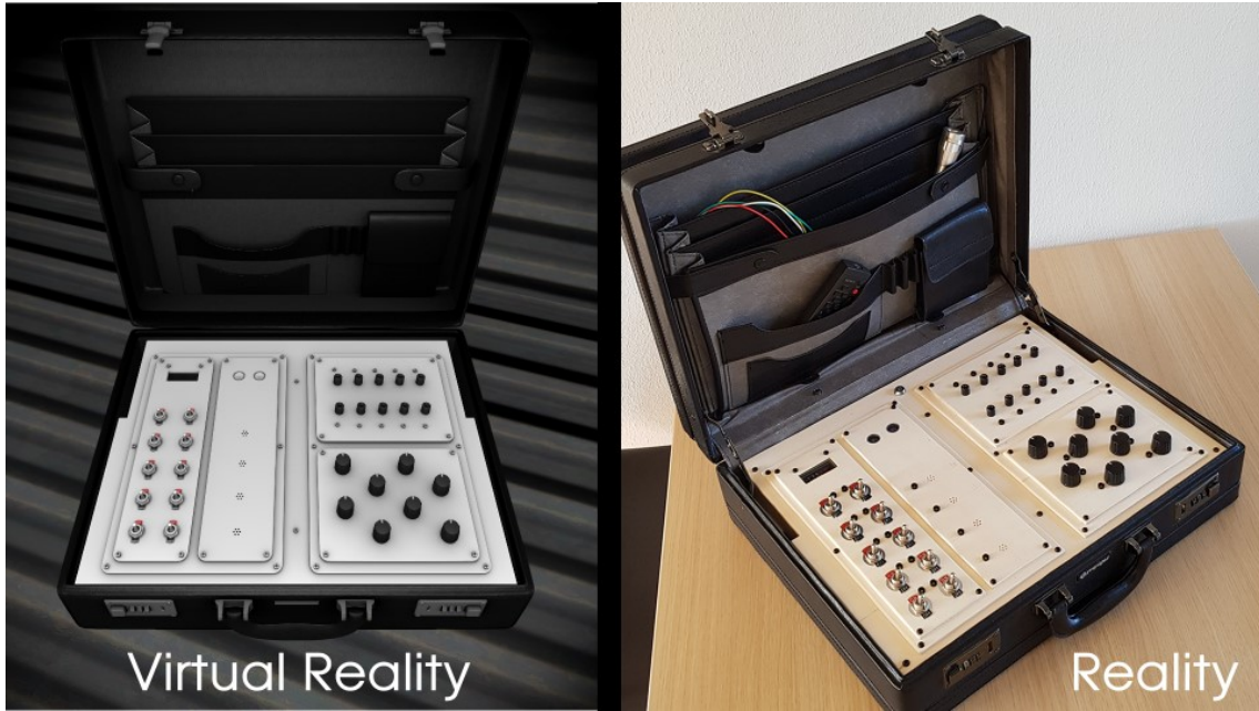
Figure 3.2.: Left: View of the digital twin for the remote expert in VR. Right: Physical "machine" seen by the local worker. The expert sees the target states and positions of the elements and can turn on and off LEDs in VR that are synchronized with the real counterpart for the local worker. Fig. from [Lad+19].
