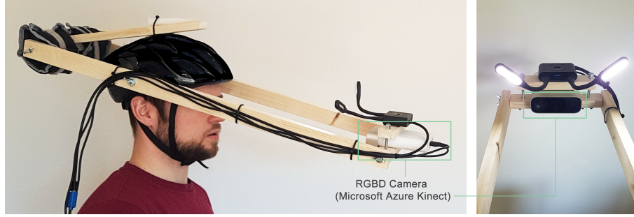
Figure 7.3.: A low-cost helmet mount helps reduce variance in the data set, resulting in shorter training times, smaller neural networks, and higher reconstruction quality. Image from [Lad+25; Lad+20b; LPG20].
