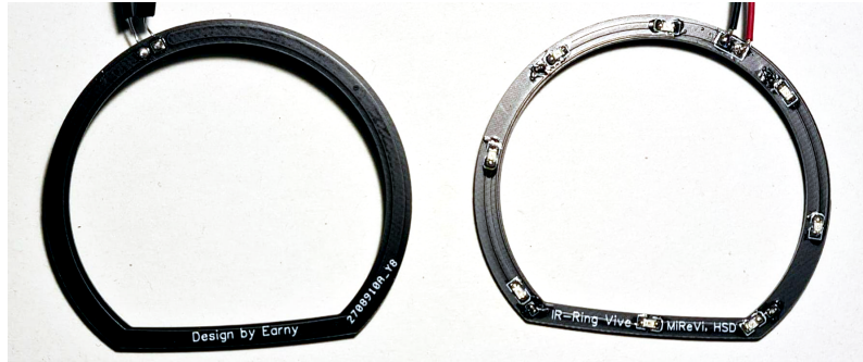
Figure 5.25.: Final IR LED ring prototype. PCB design by Bernhard "Earny" Wohlmacher.
