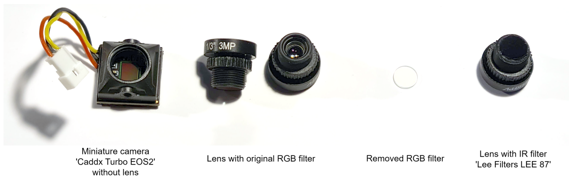
Figure 5.5.: The RGB filter was removed and a IR filter, that passes light above 730nm, was inserted.
