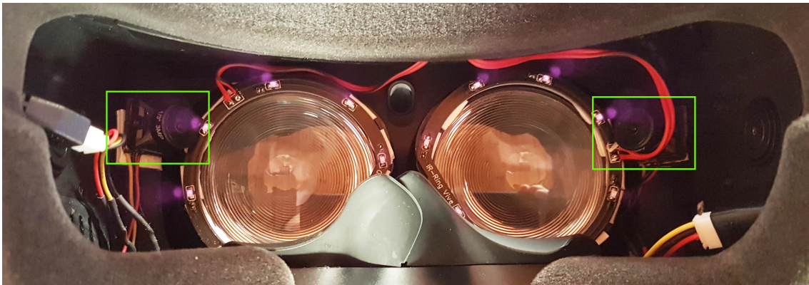
Figure 5.26.: The second prototype of the IR-LED ring circuit boards is mounted around the Fresnel lenses. For eyebrow tracking, two cameras were mounted inside the HMD, as highlighted by the green frames.
