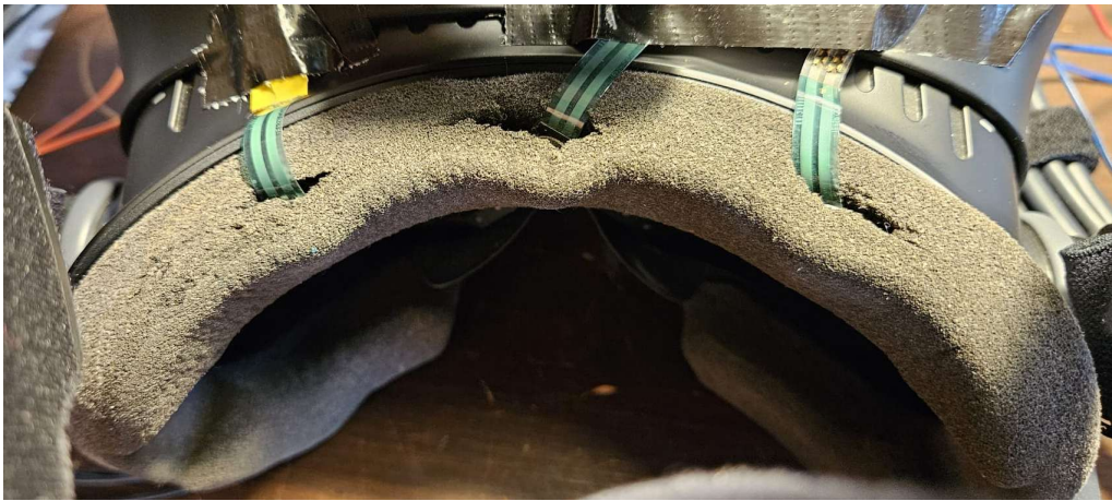
Figure 5.18.: Position of the pressure sensors in the preliminary study. Slits were cut into the foam of the HMD frame and three sensors were glued into them.
