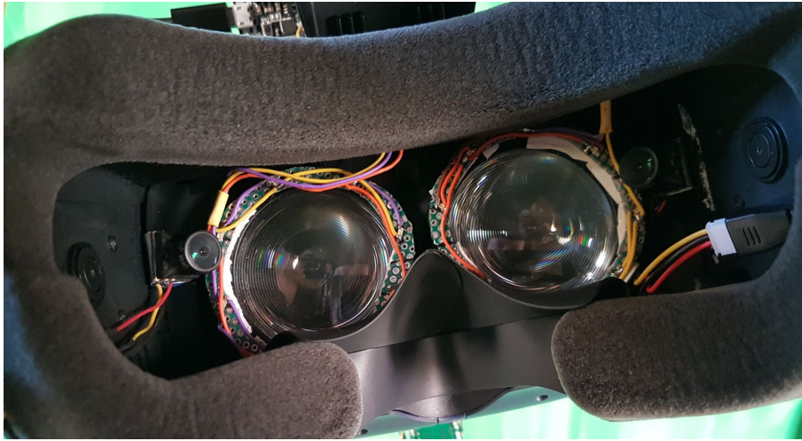
Figure 5.24.: First IR-LED-ring prototype built into the HMD. HMD is a off-the-shelf HTC Vive v1. Image credits by Juan Schupp.
