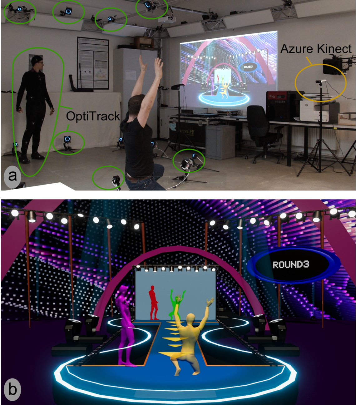
Figure 4.9.: Playing "Human Tetris" with the MotionHub. a) shows the physical set-up with OptiTrack and Azure Kinect. b) shows our evaluation game created in Unity 3D. Figures from [Lad+20a].
