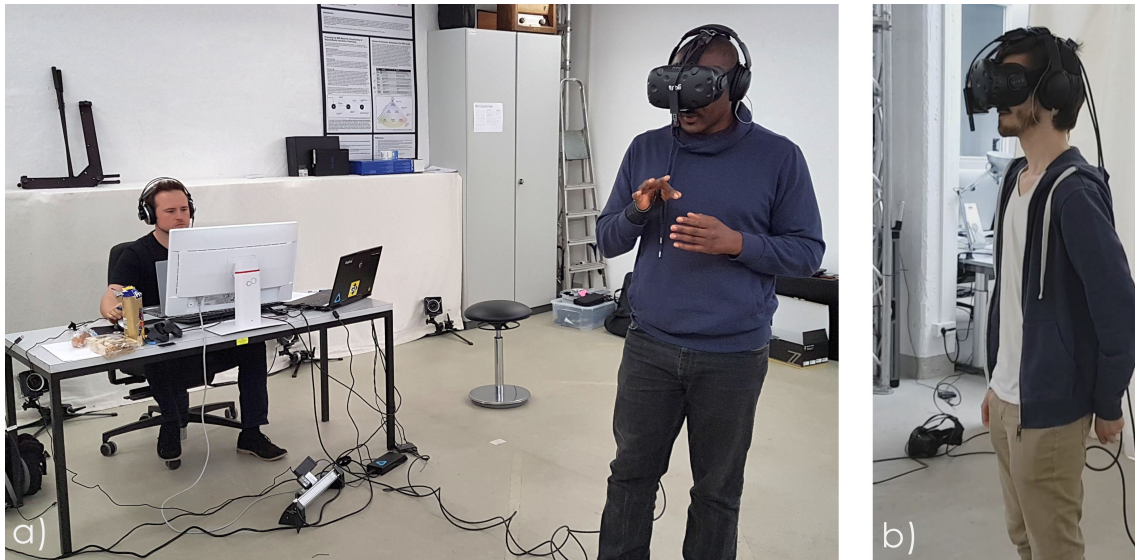
Figure 6.4.: Study setup; a) Participant wears HTC Vive with eye and lip tracking and speaks remotely with a person in another room. The experimenter at the table observes the experiment; b) The participant in another room listens while the remote person speaks. Image from [LG19b].
