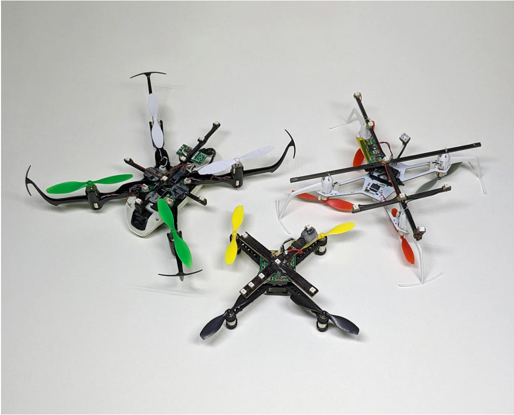
Figure 3.8: Initially, off-the-shelf hobby drones were tracked and controlled in the ICARUS testbed using prototype tracking markers.
