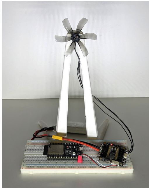
Figure 3.23: Prototype of a downwash generator to improve immersion in virtually conducted HDI user studies.
