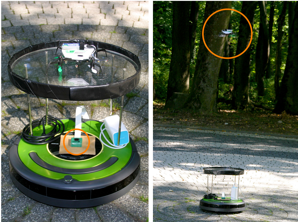
Figure 3.26: Collaboration between a mobile ground robot and a UAV. The left image shows the setup before take-off. A Raspberry Pi equipped with the Raspberry Pi camera module (indicated by an orange circle), is employed for optical pose estimation. It tracks the marker mounted to the bottom of the drone through an acrylic pane, which serves as a landing platform. In the image on the right, the hovering drone (circled) transmits images from an onboard camera to a computer for further processing.
