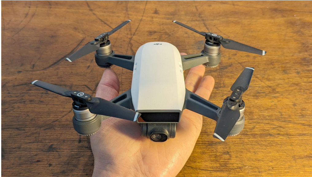
Figure 1.8: The DJI Spark is a consumer drone with a 175 mm wheelbase, which can be deployed from the operator's hand and controlled using gestures.
