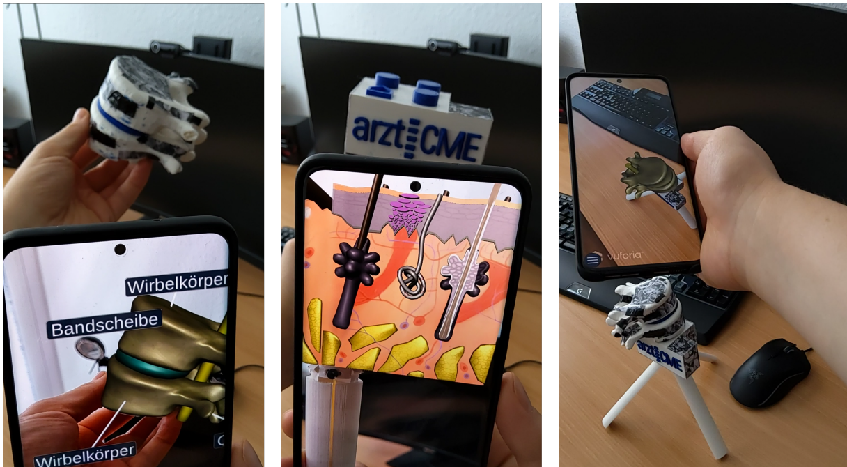
Figure 4.5: Prototype with the realistically shaped tangible interface (left), the generic tangible interface (middle), and the plug connection system interface (right).
