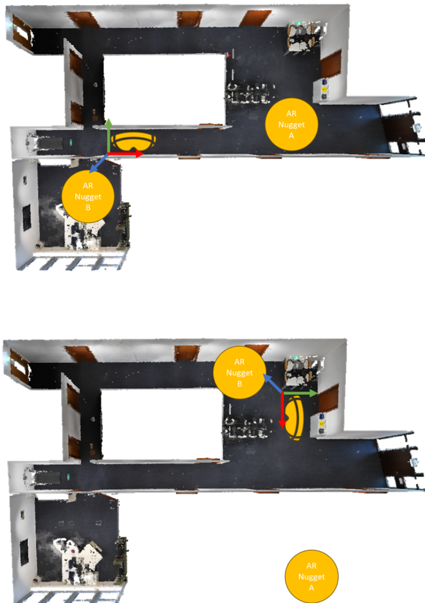
Figure 5.9: Influence of the AR device's position and rotation on application start. Top: AR Nuggets are located in the building as the author intended. The coordinate system's origin is close to the room in the lower left corner. Bottom: The application was started while the AR device was not located where the intended origin of the coordinate system is. The AR nuggets have the correct position in this coordinate system but are not correctly placed in the building.
