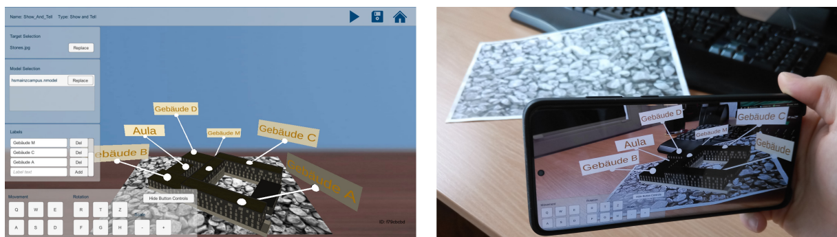
Figure 5.4: A show & tell AR nugget that was adapted using the ARNAUDDI by a person without programming knowledge. Left: Screenshot from ARNAUDDI executed on a desktop device. Right: Picture with ARNAUDDI running on the HHD. [Rau+22b].
