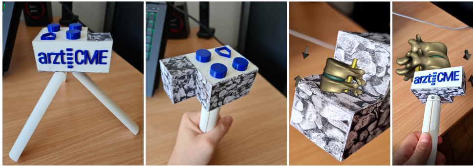
Figure 3.4: Images of our generic tangible. From left to right: 1) rested on its tripod, 2) held using its handle, 3) augmented with a virtual 3D model of vertebrae on one side that is used as a stage, 4) occluding a part of the virtual vertebrae 3D object.
